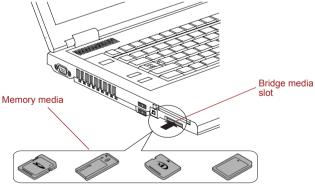
Figure 3-4 Inserting memory media
